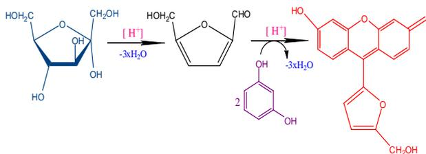
Fig. 4 Scheme of Selivanoff reaction
