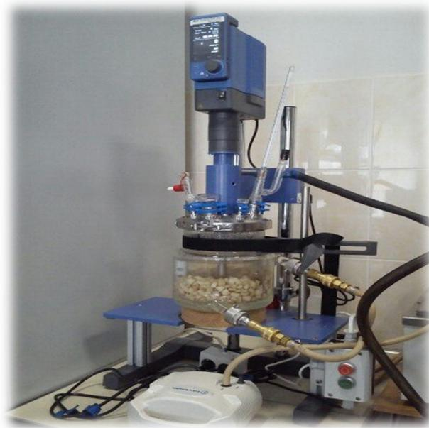
**Figure 2.** Vacuum equipment for extracting IKA EUROSTAR 200P4 control.
