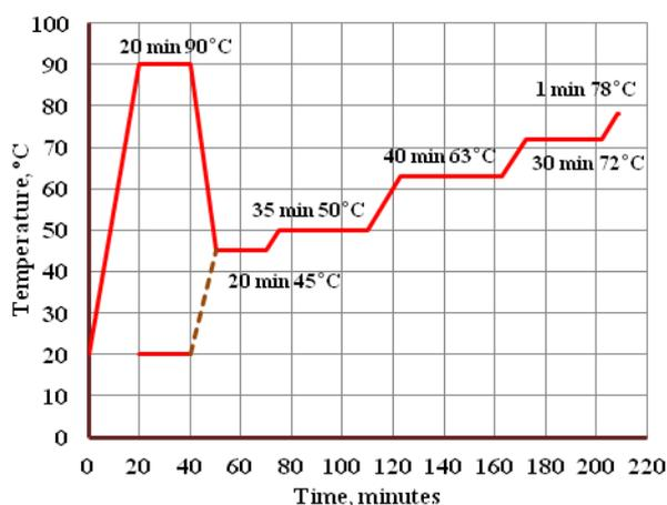
**Figure 1.** Combined decoction mashing method
