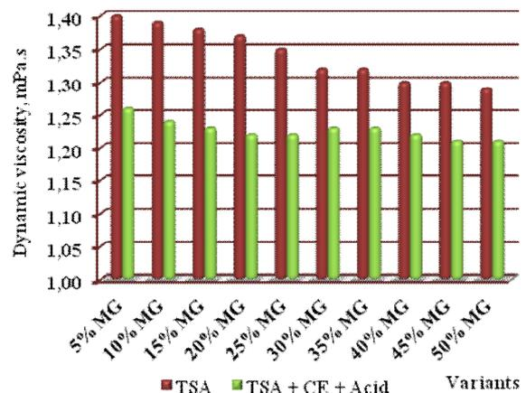
**Figure 4.** Changes of dynamic viscosity of the wort
