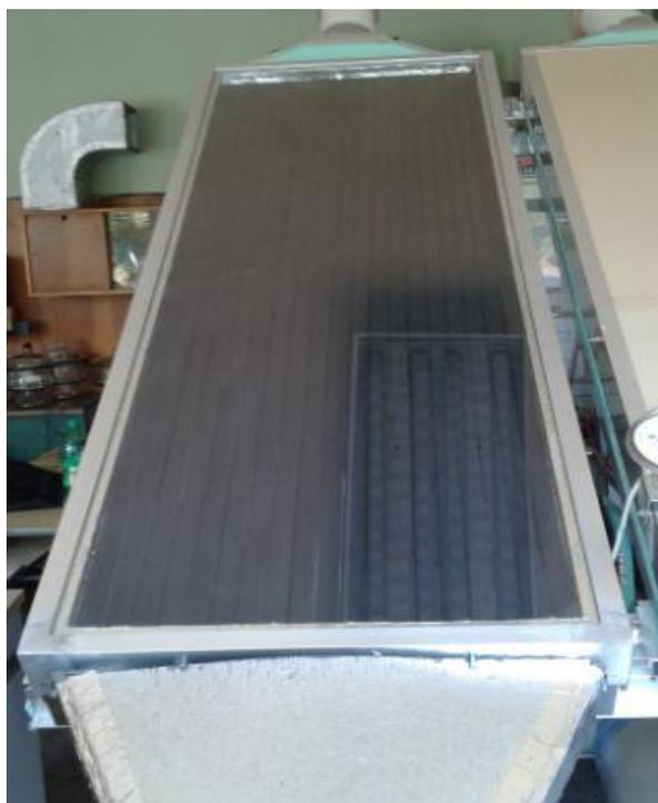
**Figure 5.** The experimentally tested air solar collector.
