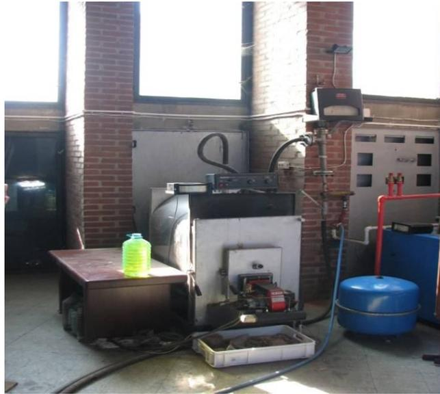
**Figure 1.** The experimental pilot boiler, mounted to the water delivery system and to the flue gas evacuation
