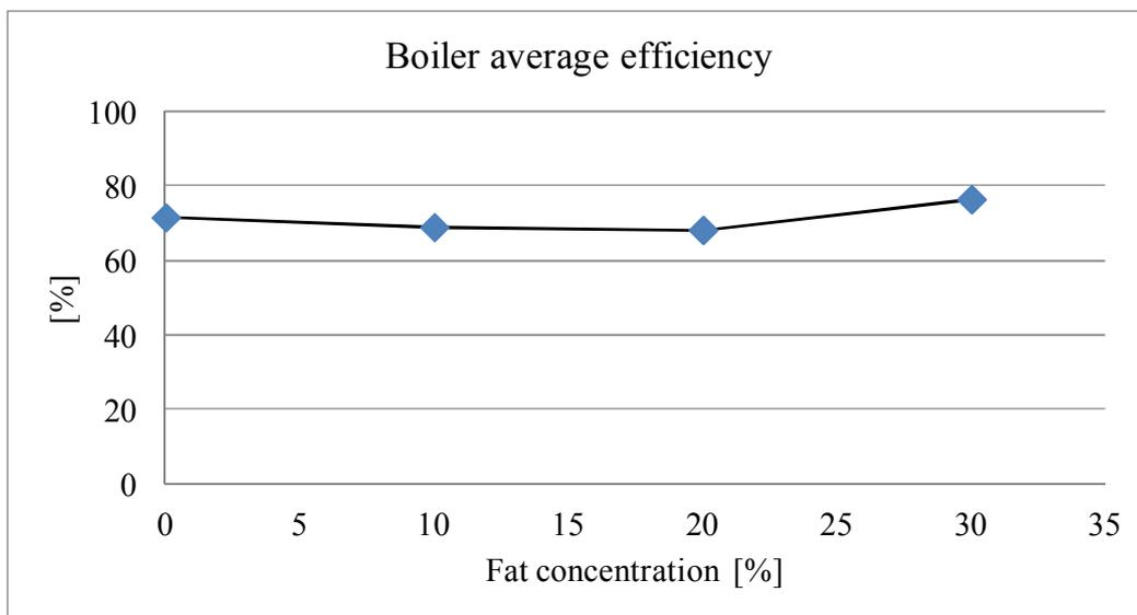
**Figure 7.** Boiler efficiency variation as a function of the animal fats concentration in the fossil liquid fuel
