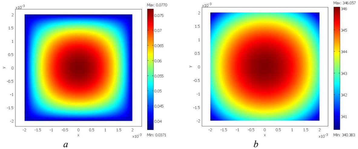
**Figure 1.** Moisture content (a) and temperature (b) fields at the instant of time  $t = 2700$  s
