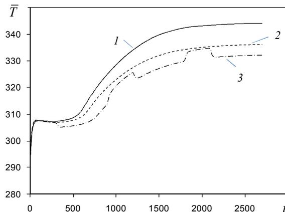
*1* – mode 1 with constant microwave field intensity and  $\epsilon'' = \text{const}$ ; *2* – mode 1 with constant microwave field intensity and  $\epsilon'' = 3,4u + 4,6$ ; *3* – mode 2 with impulse microwave action and  $\epsilon'' = 3,4u + 4,6$
