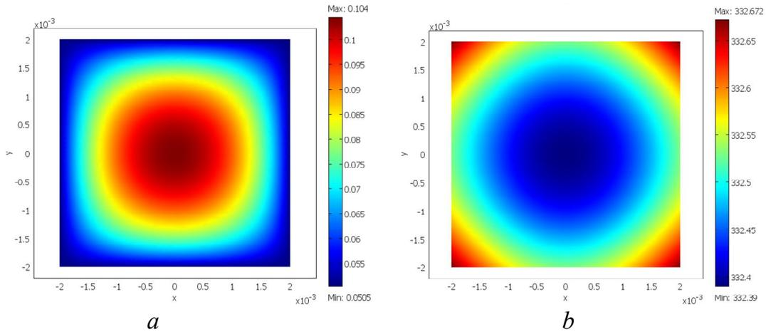
**Figure. 3.** Moisture content (a) and temperature (b) fields at the end of the process at  $t = 2700$  s and mode 3 with impulse microwave field intensity
