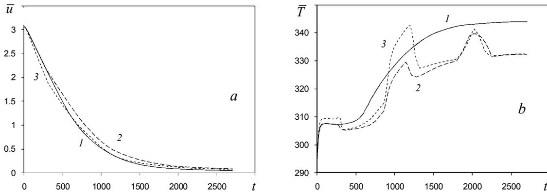
*1* – mode 1 with constant microwave field intensity; *2* – mode 2 with impulse microwave action;
